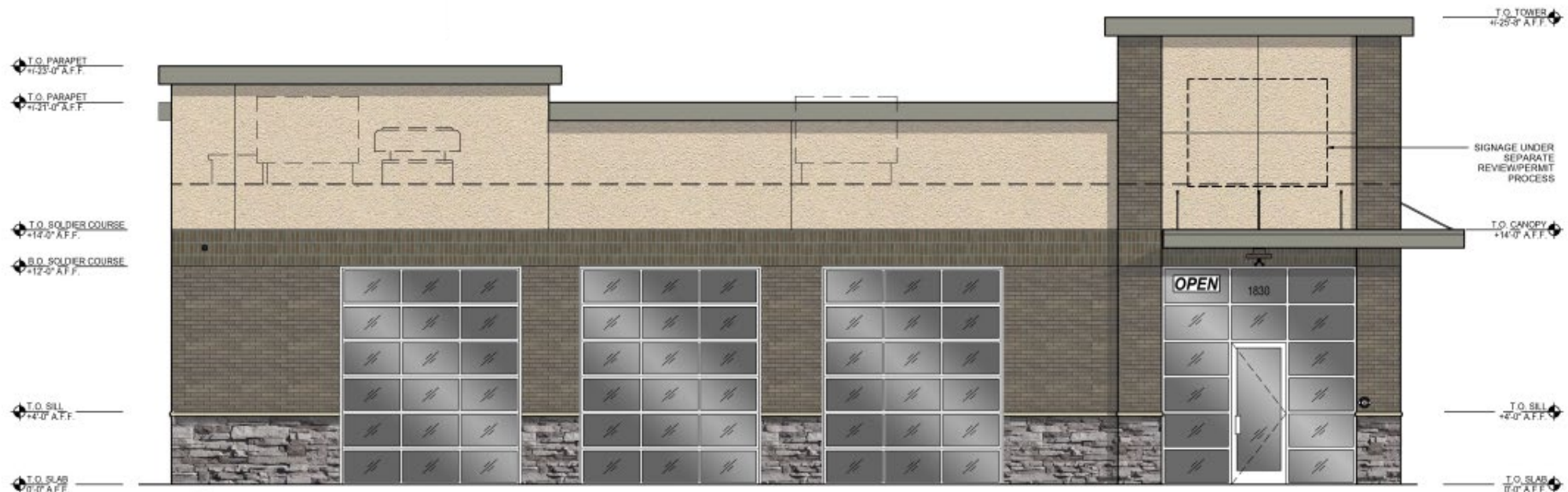
3 FRONT ELEVATION STONE / BRICK / EIFS
