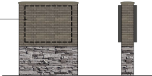
5 MONUMENT SIGN ELEVATIONS STONE / BRICK / EIFS
