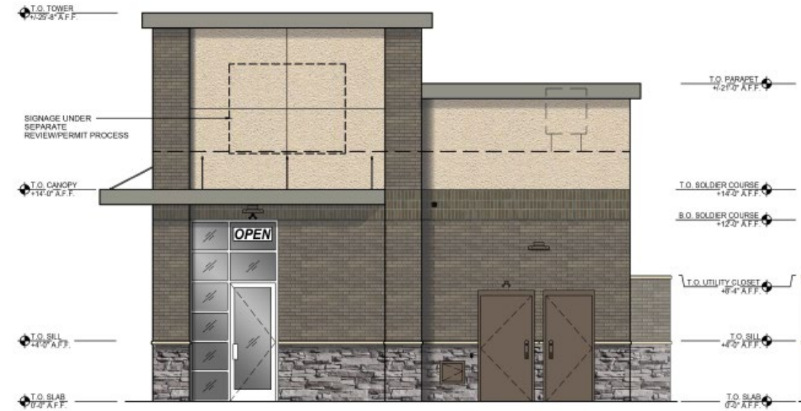
1 RIGHT ELEVATION STONE / BRICK / EIFS
